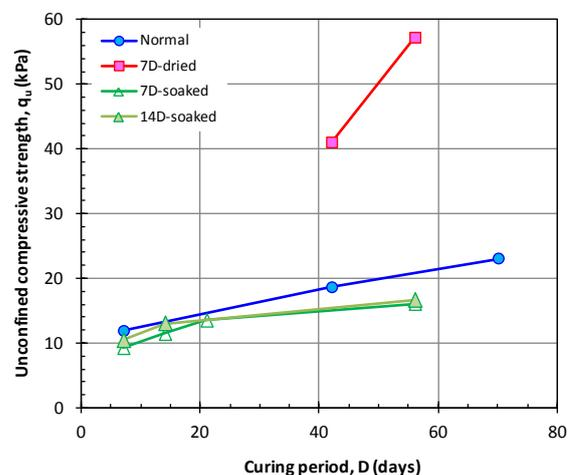
Figure 7. Effect of initial condition of slag on  $q_u$
