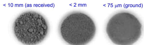
Figure 2. Steel slag - different particle sizes
