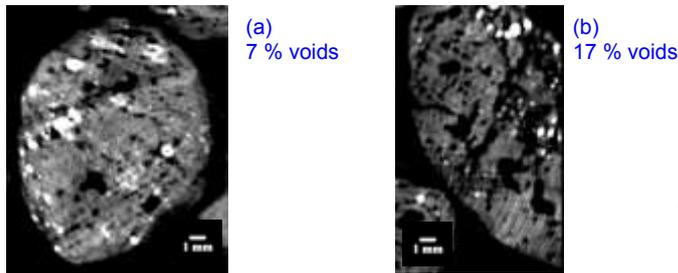
Figure 3. CT (computer tomography) images of slag particle
