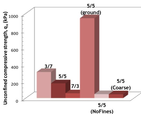
Figure 5. 28-day strength of specimens with 1.5LL and various C/S ratios
