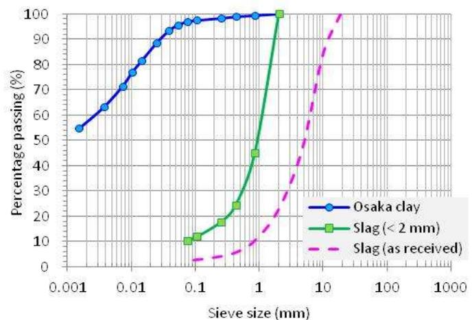
Figure 1. Particle size distribution of clay and slag
