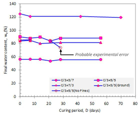
Figure 6. Water content change with time (1.5LL specimens)
