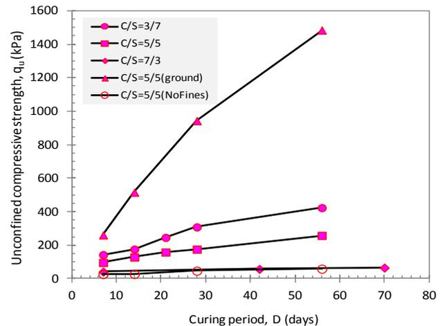
Figure 4.  $q_u$  – curing period plot for specimens with 1.5LL mixing water content
