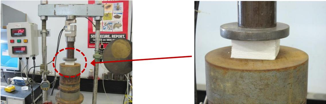
Figure 1: Polystyrene uniaxial test setup showing 50% strained position.
