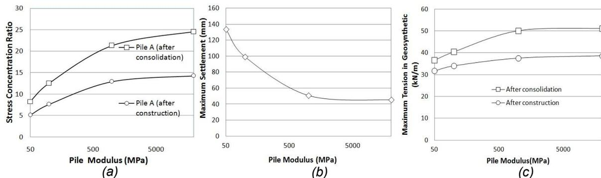
Figure 4. (a) SCR vs elastic modulus of piles (b) Maximum settlement at the embankment crest vs elastic modulus of piles (c) Maximum tension in the geosynthetic layer vs elastic modulus of piles
