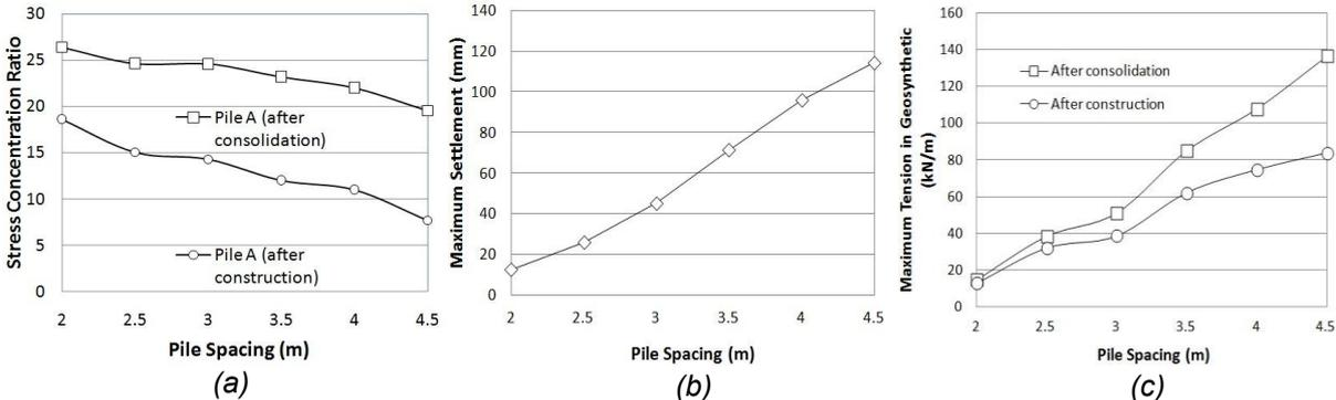
Figure 2. (a) SCR vs pile spacing (b) Maximum settlement at the embankment crest vs pile spacing (c) Maximum tension in the geosynthetic layer vs pile spacing.
