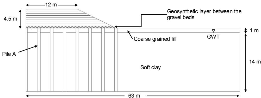
Figure 1. Cross section of the embankment with soil profile
