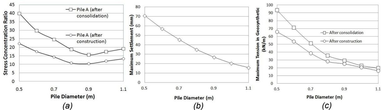
Figure 3. (a) SCR vs pile diameter (b) Maximum settlement at the embankment crest vs pile diameter (c) Maximum tension in the geosynthetic layer vs pile diameter
