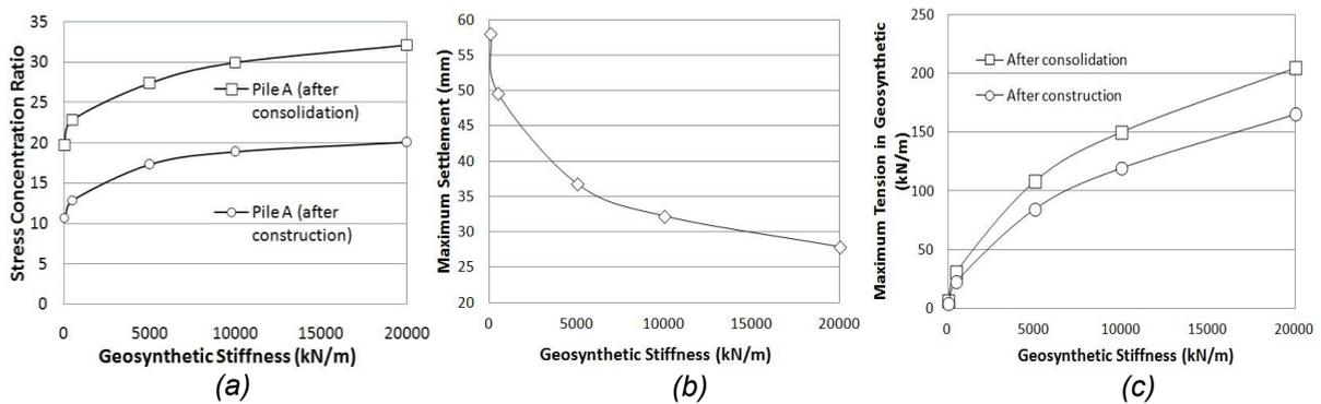
Figure 5. (a) SCR vs geosynthetic stiffness (b) Maximum settlement at the embankment crest vs geosynthetic stiffness (c) Maximum tension in the geosynthetic layer vs geosynthetic stiffness
