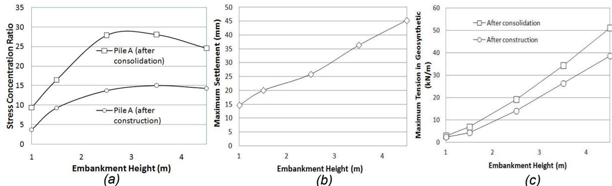
Figure 6. (a) SCR vs embankment height (b) Maximum settlement at the embankment crest vs embankment height (c) Maximum tension in the geosynthetic layer vs embankment height
