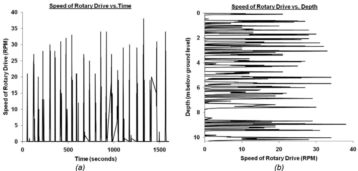
Figure 1: (a) Filtered data showing only time periods of active excavation advancement; and (b) equivalent dataset placed within a vertical excavation log, based on excavation log notes.
