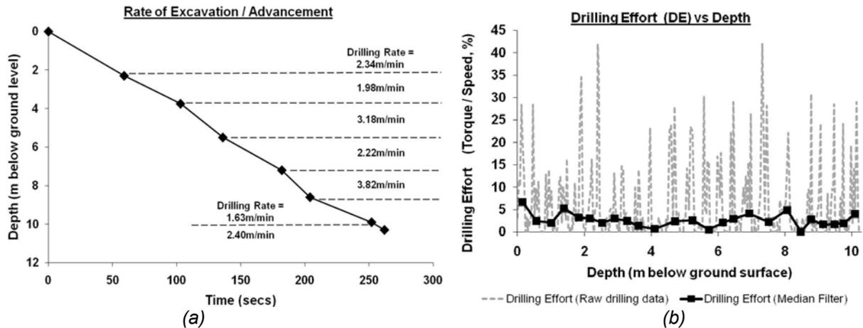
Figure 2: (a) Calculated penetration rate plotted against depth, based on piling rig data and excavation log notes; and (b) Drilling Effort, raw and filtered with median filter, plotted against depth.
