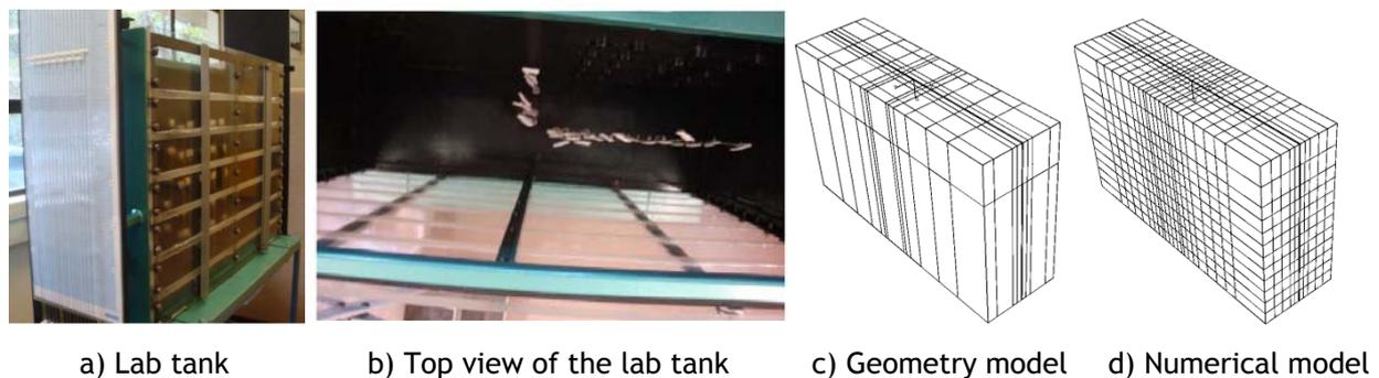
Figure 3. Finite element model for the laboratory tank consolidation experiment
