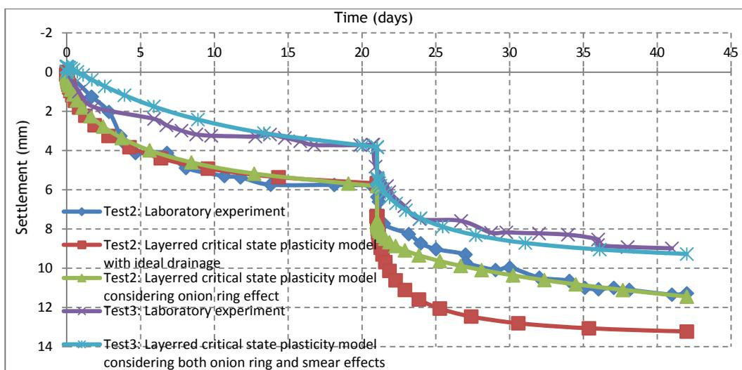
b) Test 2 and 3: consolidation tests with prefabricated and inserted, respectively wick drains
