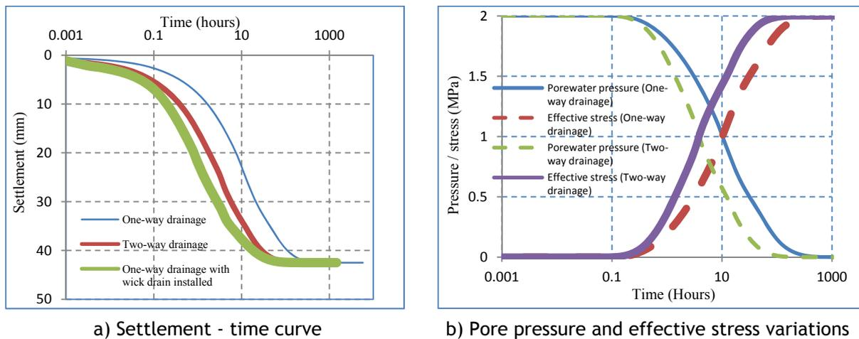
Figure 2. Modelled results of 1D soil consolidation using the pore-fluid and stress coupling method
