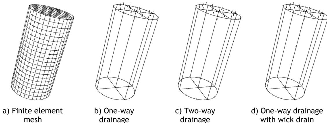
Figure 1. Numerical model showing the finite element mesh, drainage and surcharge
