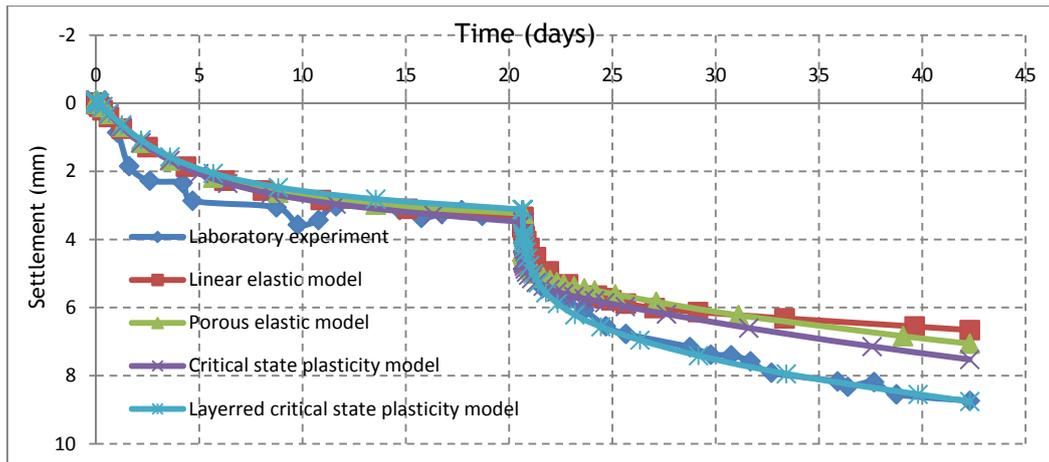
a) Test 4: consolidation test with 10 mm water layer at top drainage surface
