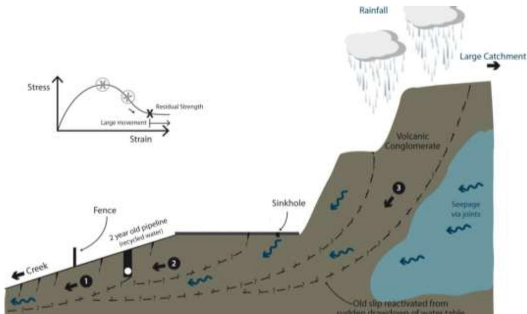
Figure 1 Pipeline located down-slope of road with active landslide
