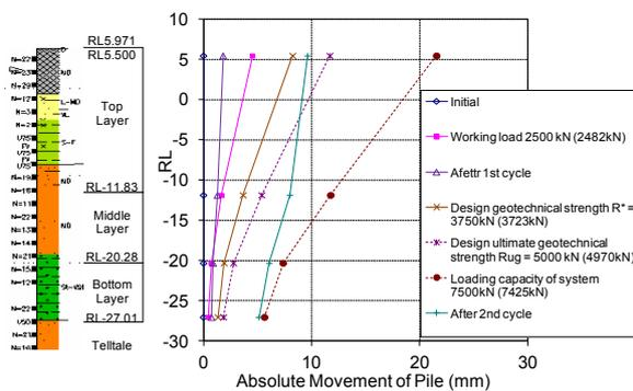
Figure 7. Absolute movement of pile under various load conditions
