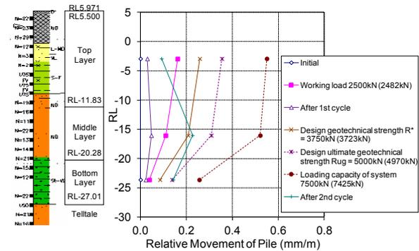
Figure 8. Average movement of pile under various load conditions
