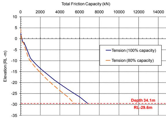
Figure 6. Test pile (with mass for soil plug) total friction capacity
