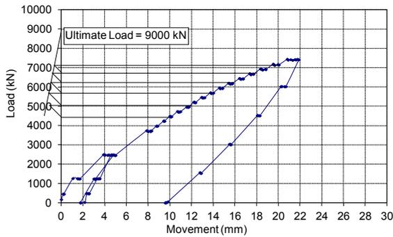
Figure 5. Prediction of ultimate geotechnical strength in tension (Mazurkiewicz's method)
