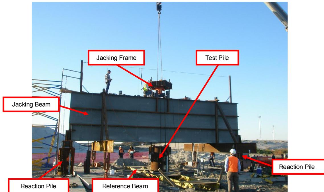
Figure 1. Overview of pile load tension test
