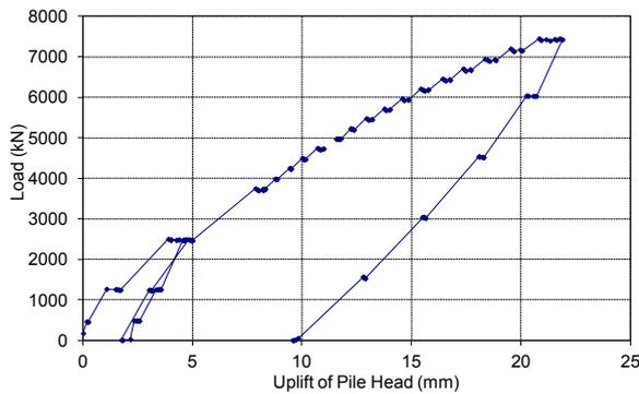
Figure 3. Load versus uplift of pile head
