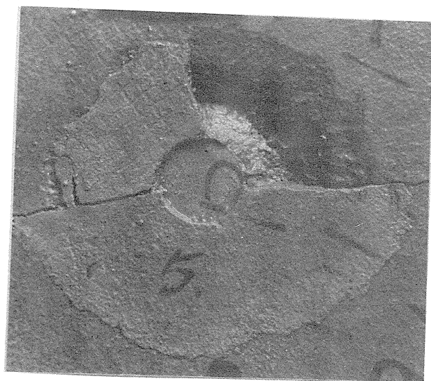
Fig. 1 Development of tension cracks in model footing test on soft rock
