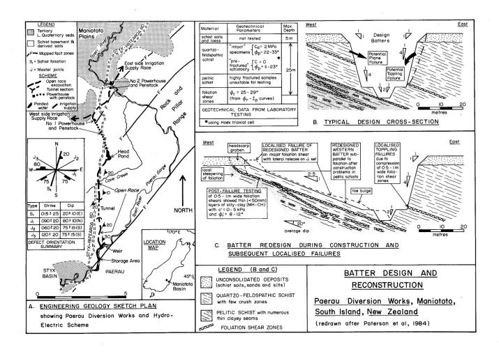
FIG 2: Batter Design and Reconstruction for the Paerau Diversion Works, Maniototo
