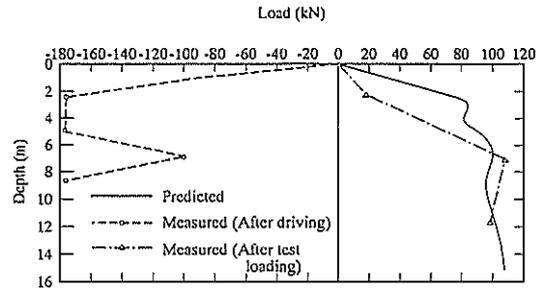
FIG.6 PREDICTED RESIDUAL LOAD DISTRIBUTION FOR DRIVEN STEEL TUBE PILE
