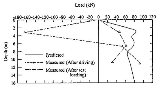
FIG.7 PREDICTED RESIDUAL LOAD DISTRIBUTION FOR DRIVEN H-PILE
