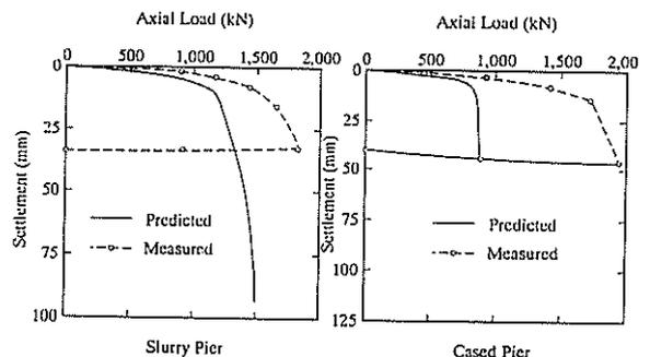
FIG.3 PREDICTED AND OBSERVED LOAD-SETTLEMENT OF BORED PILES
