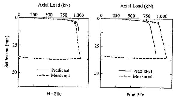
FIG.2 PREDICTED AND OBSERVED LOAD-SETTLEMENT OF DRIVEN PILES
