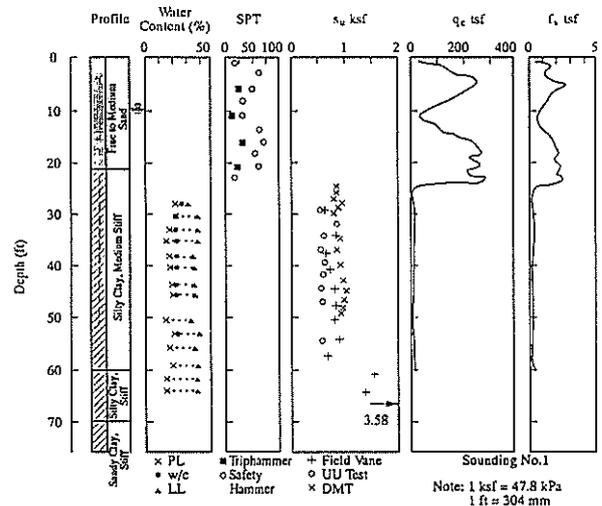
FIG.1 SUMMARY OF GEOTECHNICAL PROFILE AND DATA PROVIDED
