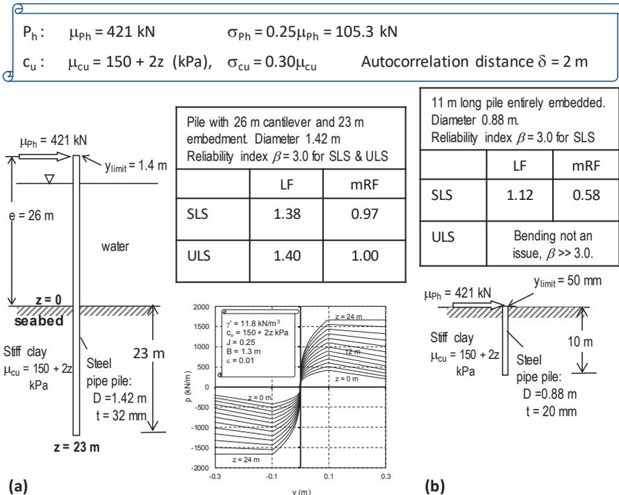
SLS = Serviceability limit state, pile head deflection  $y_{limit}$
