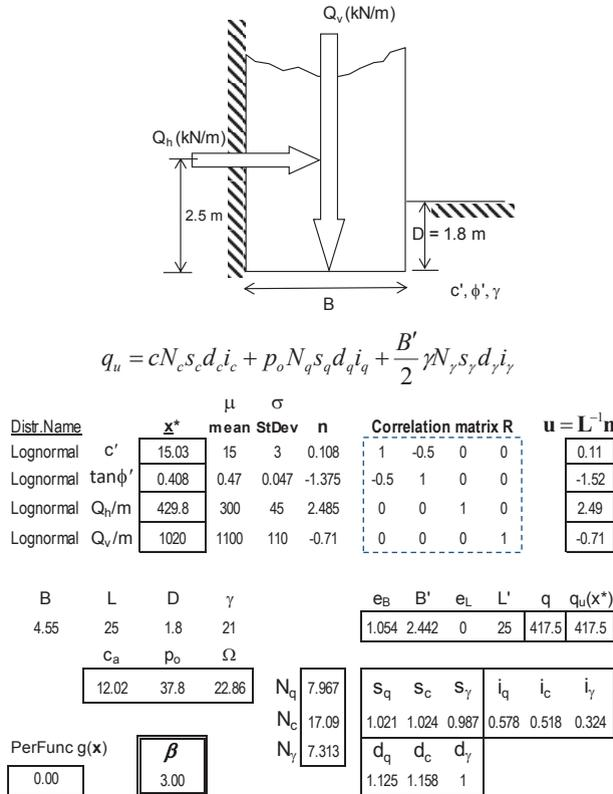
**Figure 2.** RBD-via-FORM for the width B of a spread footing. The vertical load  $Q_v$  possesses stabilizing-destabilizing duality when horizontal load  $Q_h$  is acting.
