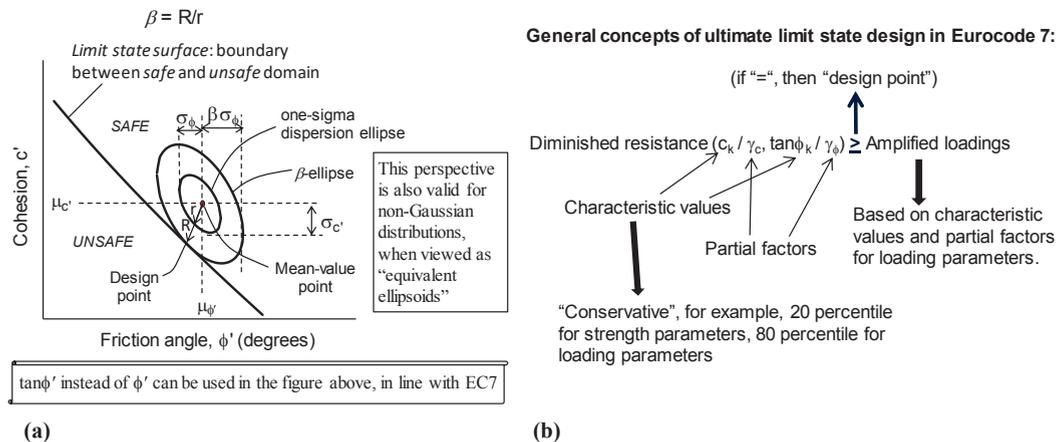
**Figure 1.** (a) FORM design point reflects parametric correlations and context-sensitivities; (b) EC 7 design point based on conservative characteristic values and code-specified partial factors.
