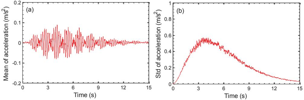
Figure 2. An example of mean (a) and standard deviation (b) of seismic ground motion.
