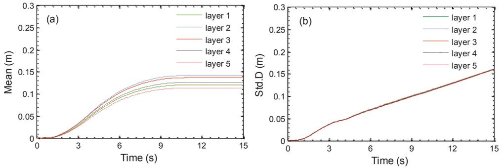
**Figure 4.** The mean value (a) and standard deviation (b) of the horizontal displacement of the slope face at different reinforcement elevations.
