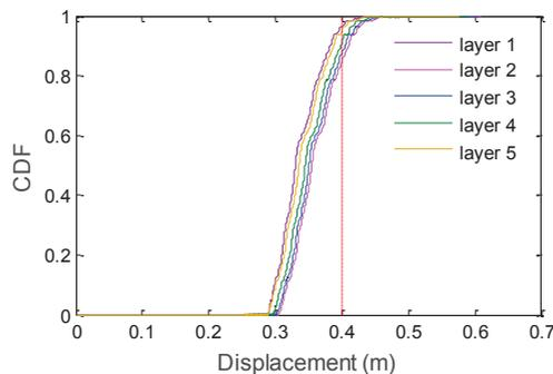
**Figure 6.** The CDF of the maximum horizontal displacement of the reinforcement soil slope at different reinforcement layers.
