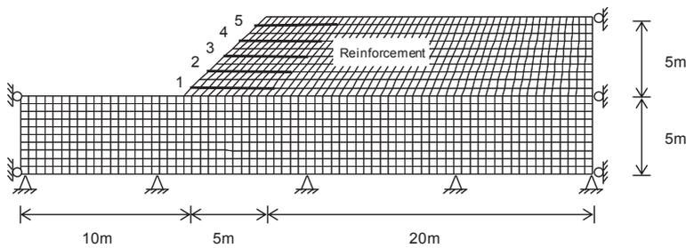
Figure 3. The geometry of reinforcement soil slope.
