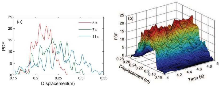
**Figure 5.** The PDF of the horizontal displacement of the slope face at the second reinforcement layer: (a) for three discrete times and (b) between 4-5s.
