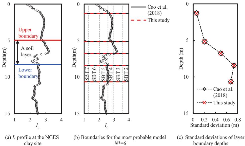
Figure 1. Comparison of soil stratification results with those in Cao et al. (2018).
