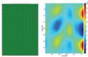
Figure 6. FE model and random field sample.
