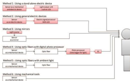
Figure 1. Various methods for monitoring and data visualization.
