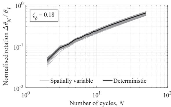
Figure 5. Normalised accumulated rotation at the mudline in spatially variable clay.
