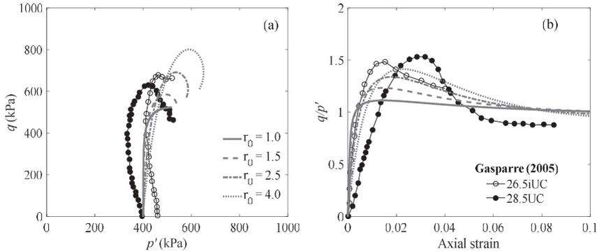
**Figure 1.** KHSM predictions and laboratory data for undrained triaxial compression tests on London Clay: (a) stress path; (b) stress-strain response.
