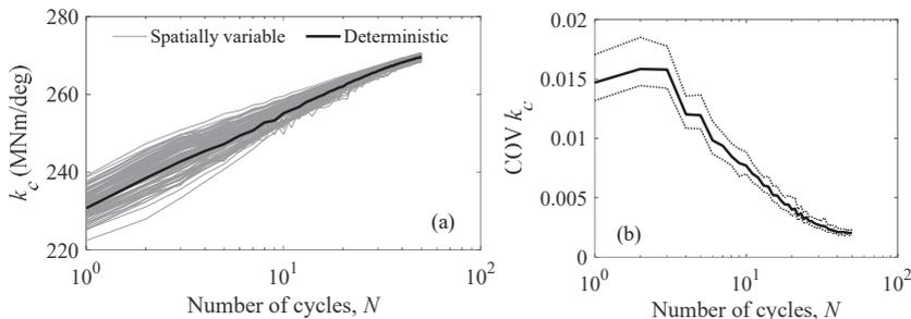
Figure 6. (a) Cyclic secant stiffness,  $k_c$ , in spatially variable clay; (b) COV of  $k_c$  (dotted lines show 95% CI).
