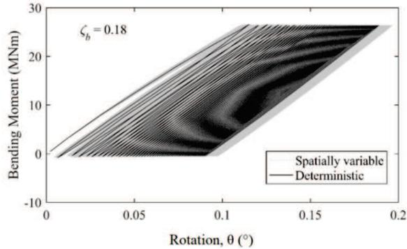
Figure 4. Bending moment - rotation of the monopile at the mudline.
