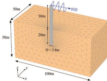
Figure 2. Finite element mesh.
