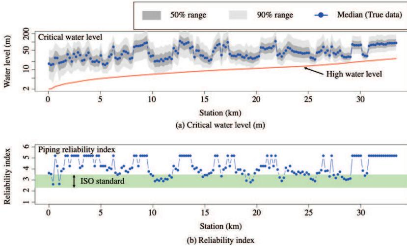
Figure 2. Reliability analysis results assuming to be conducted soil investigation at 200m intervals
