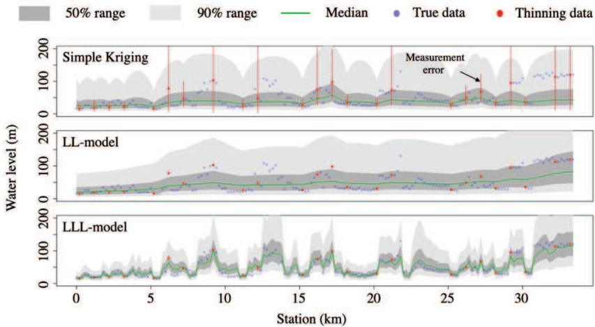
Figure 3. Estimation result of critical water level in each model
