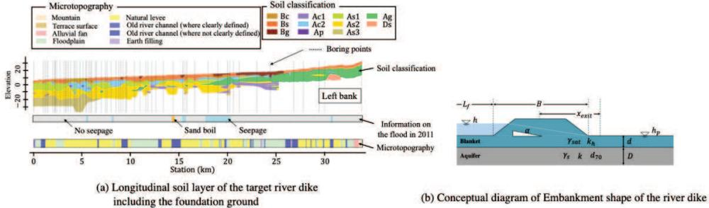
Figure 1. Soil investigation data in the target river dike using calculation
