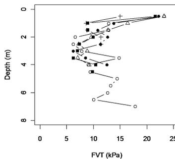
**Figure 2.** Undrained shear strength of the topsoil
